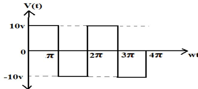
3. a) Find the Trigonometric Fourier series for the following waveform shown in figure. [5M]
