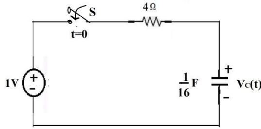
2. a) Derive the Transient Response of series RC-circuit with D.C excitation. [5M]
